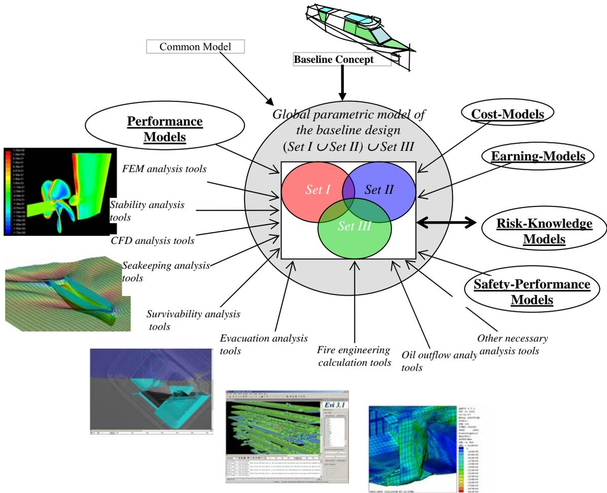
Figure 20: Concept for integration of PERC knowledge models [key parameters + prediction models] with performance and safety-performance analysis tools within a ship design optimisation environment
