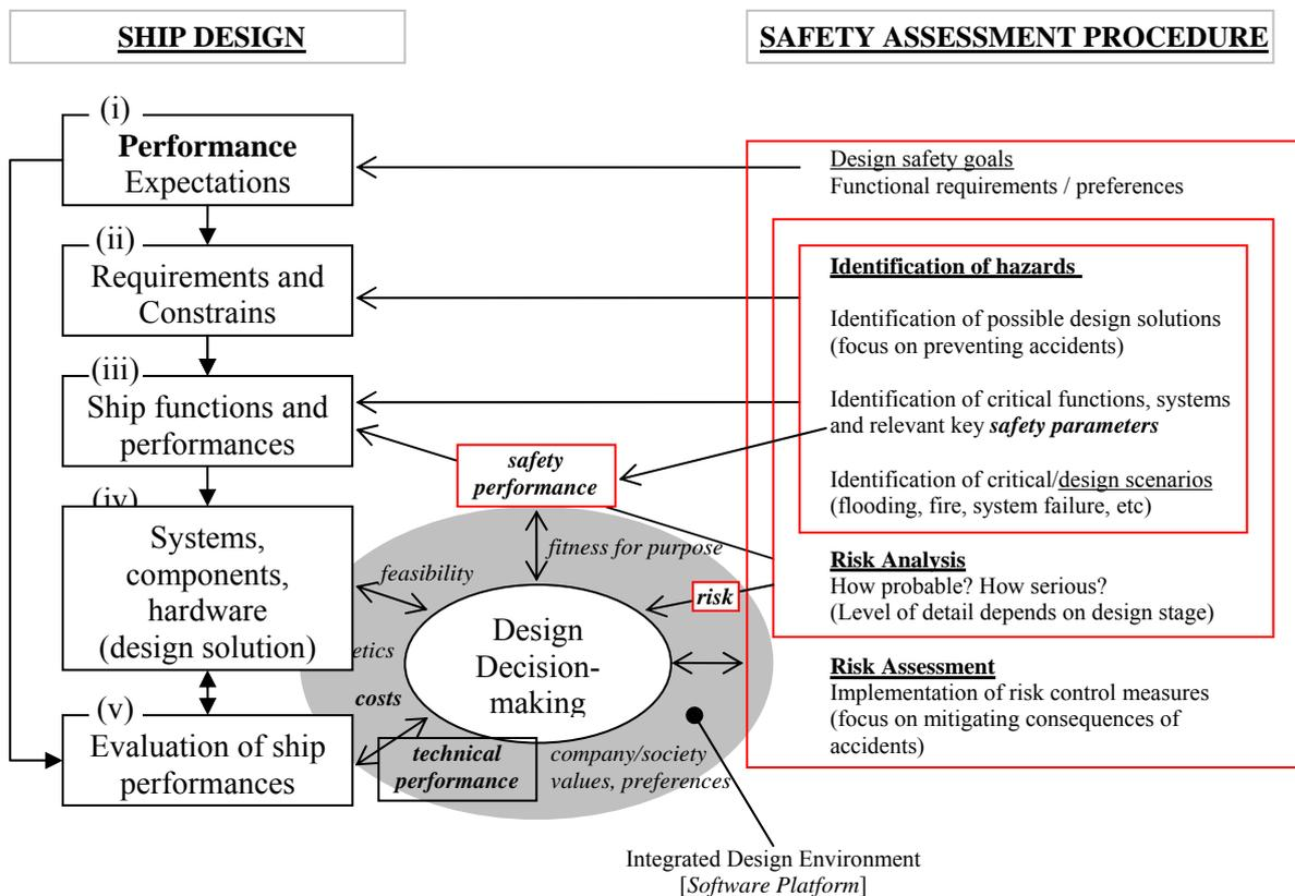
Figure 15: A high-level framework for risk-based design implementation
