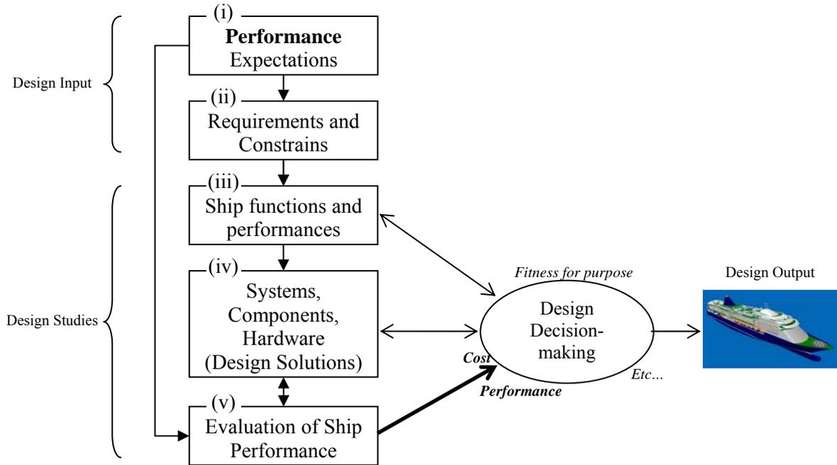
Figure 14: High-level conventional design process
