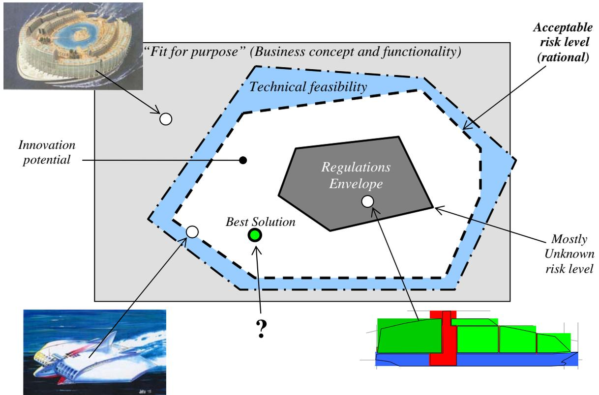
Figure 21: Possible design solution envelopes
