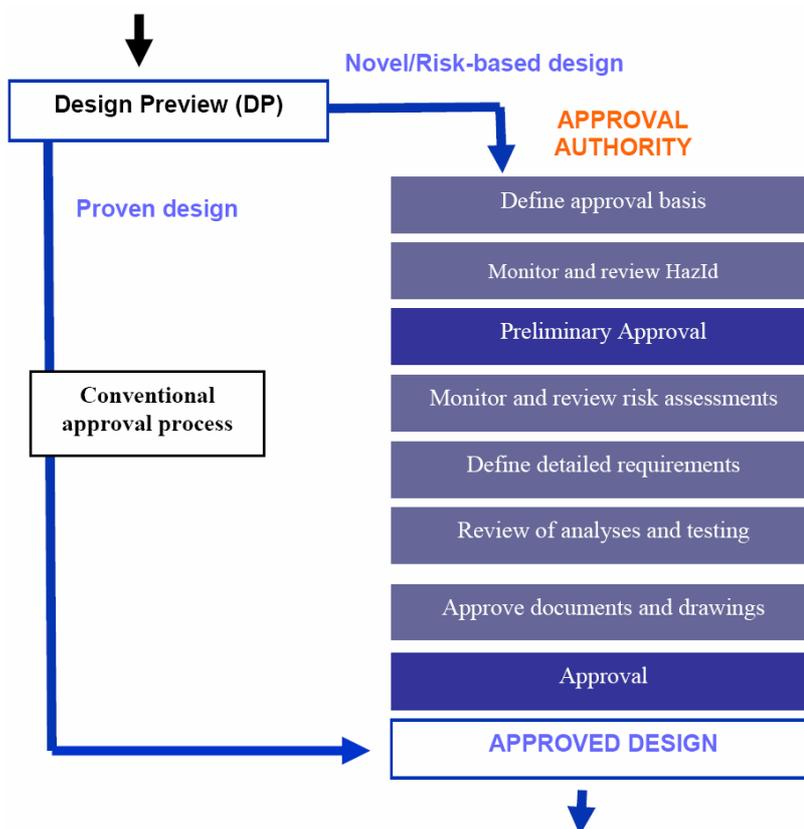
Figure 13: High-level approval process for novel and risk-based design
