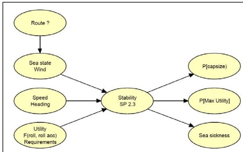
Figure 8: Interaction diagram for SP2.3
